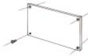
36 —Drilled, with Countersunk Phillips Screws
