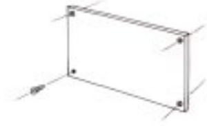
37 —Drilled, with Clutch Head Screws
