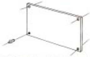
38 —Drilled, with Drive Rivet Fasteners
