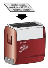
**Step 4.** Apply the rubber die to the adhesive coated die plate <u>as illustrated.</u>
