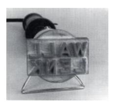
Letters fit into a slot(s) in the branding head and can be interchanged. Heads with one or two slots are available. Letter sizes offered are 3/16", 1/4", 3/8", 1/2", 3/4", and 1 inch high. Some sizes can be intermixed on a head. Screw held End Locks hold letters securely in slot.
