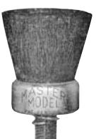
The BRUSH TIP is manufactured with top quality black hog bristle of the proper stiffness for fast stenciling and long wearing quality. The bristles are set in vulcanized rubber, further secured with a crimped brass ferrule finished in nickel plate. The construction of the brush tip is patented under Patent Nos. 2164004 & 2235734.
