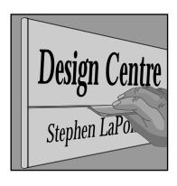
**1.** Using the "Multiple" side of the NEXUS Key, insert at right angles between two FacePlates and push in as far as possible.
