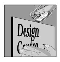
**1.** Place either "Single" corner of the NEXUS Key against the wall, insert the sharp corner between the FacePlate and MountPlate and push in.
