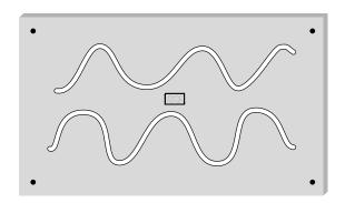
Apply a 1/4" wide continuous bead of silicone adhesive in a diagonal serpentine course. Maintain a 1/2" clearance from the edge of the sign.
