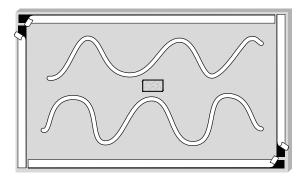
Apply a 1/4" wide continuous bead of silicone adhesive in a diagonal serpentine course. Maintain a 1/2" clearance from the foam adhesive.
